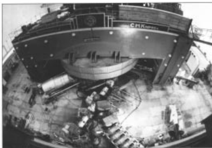
Fig. 5: Phasotron with space variation of the magnetic field, proton energy (660 \pm 3.1) \text{ MeV} , extracted beam intensity 3 \times 10^{13} \text{ p/s} , duty cycle - 85%
