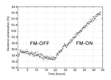
The plot shows the build-up of deuteron polarization in LiD over time with and without FM
