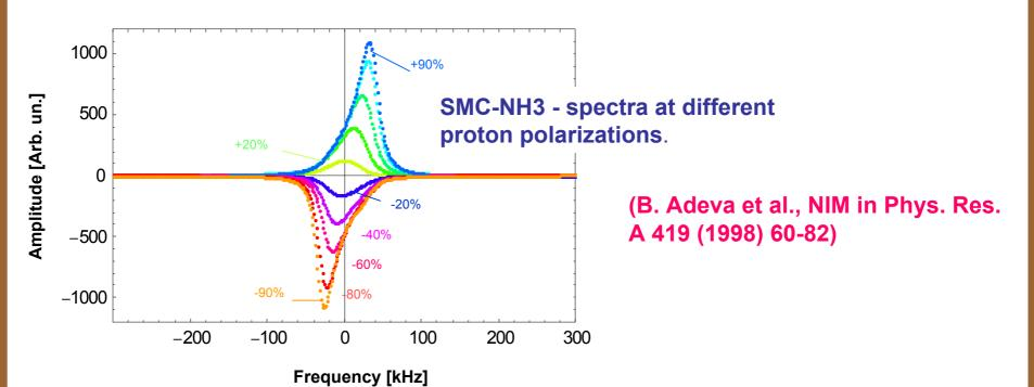
Our studies show that the signal asymmetry is proportional to the proton polarization. This allows to determine the proton polarization by the line shape of NMR-spectra.
