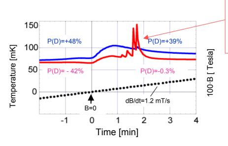
Here you can see the coherent radiation of D and Li<sub>7</sub> obtained on the COMPASS polarized target at CERN
