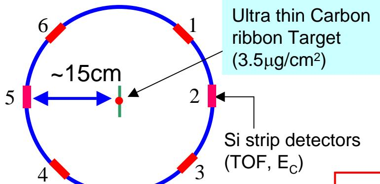
Thin dead layer for low energy carbon spectroscopy
